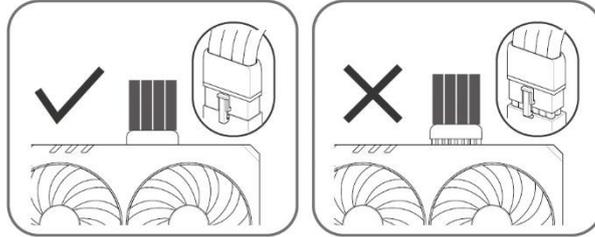
Make sure that the end of the 16-pin cable and all other cables labeled "PSU" is fully inserted into a matching port on the power supply, so that the plastic tab on the top of the cable connector clicks into place.
