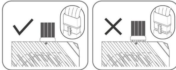
Make sure that the power supply cables labeled "PCI-E" are fully inserted into the four sockets on the adapter cable, so that the tabs on the top of the connectors click into place.
