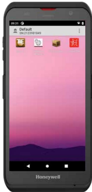
Launcher - gives the customer total control over which apps can be run on the device.
