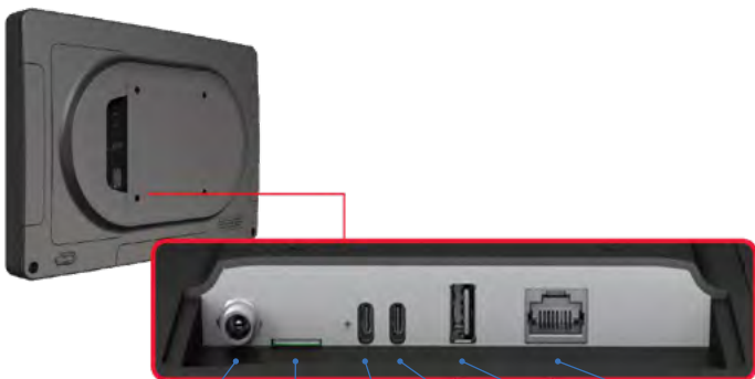
DC-IN Jack SIM USB 3.0 Host USB 2.0 OTG USB 3.0 Type-A RJ45 LAN w/POE
